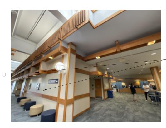
AND OAK TRIM TO REMAIN. WALL **BEHIND VALANCE** TO BE DEMO'D, PATCH AND REPAIRED AS REQUIRED.
